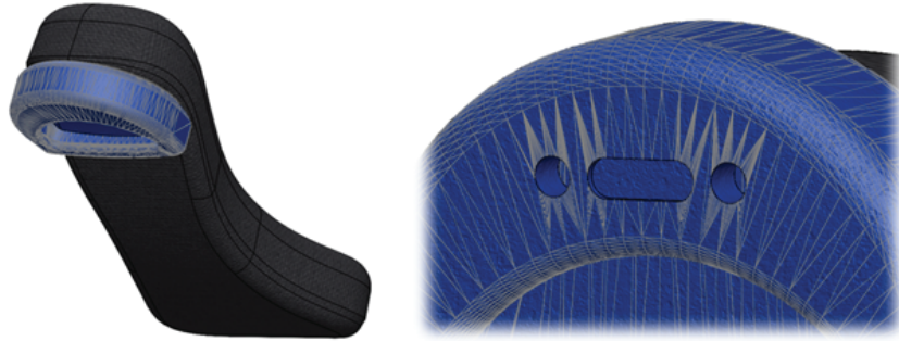
Mesh body combined with traditional SOLIDWORKS body; Extruded Cuts added
